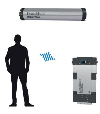
Determination sound pressure level 1m in front of dryer
