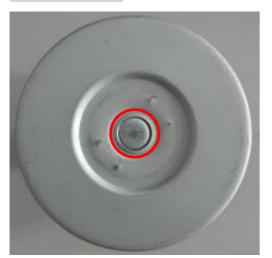
No seal, dirt particles pass the engine Small opening, inefficient oil flow Too low opening pressure, no filtration
