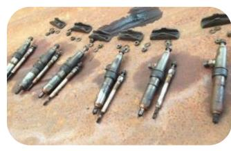
Damaged fuel injector
