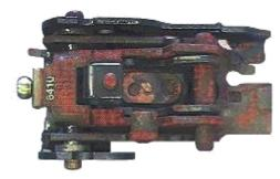
Parts corroded by water contaminated fuel
