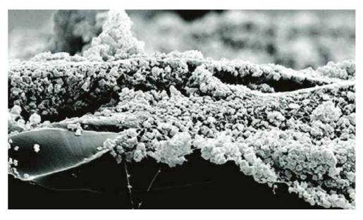
Nanofibre media is loaded with ISO fine dust. Dust particles collect on the surface of the media and vibrate off with equipment use – allowing the filter to last longer.
