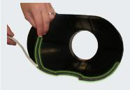
Push the PowerCore® inlet adapter over the end of the air cleaner until the holes are aligned over the U clip nuts. Insert the bolts, with washers, into the holes and tighten gently.
