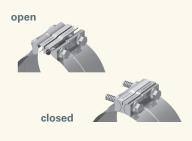
Note: Do not exceed 70 ft. lbs. torque as clamp damage may occur.
